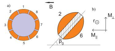
*Fig. 1* - a) Schematic drawing of the Gundestrup probe b) Vector convention used
