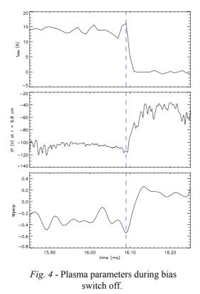
As the bias voltage is switched off the decay time of both the electric field and poloidal flow is roughly ~15  $\mu$ s, which is much smaller than the expected damping time based on magnetic pumping mechanism (~100  $\mu$ s) and charge exchange (~500  $\mu$ s) indicating that anomalous viscosity may play an important role in edge poloidal damping.
