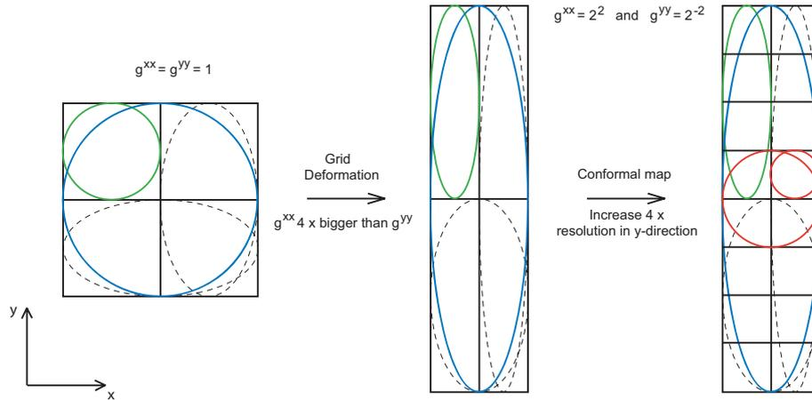
Figure 2: Illustration of the grid deformation caused by variation in perpendicular metric components, and its consequence in terms of preventing the coexistence of isotropic modes in the plane perpendicular to the magnetic field. The ultimate remedy is illustrated in the right-most figure: the conformal map.
