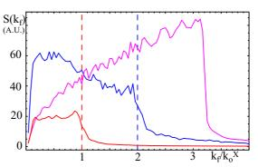
Figure 1: Phase fluctuation spectrum for O (red) and X (blue) modes on the same probed zone with the detection limits (dashed lines)
