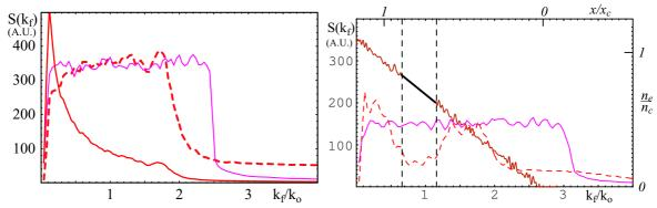
Figure 3: Phase fluctuation spectrum for Omode for parabolic density profile (red line), reconstructed density fluctuation spectrum (red dashed line) and the input (magenta).
