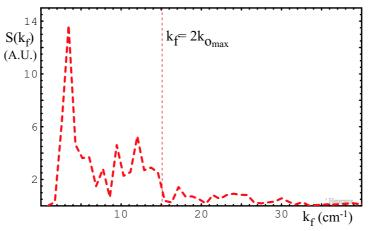
Figure 6: Reconstructed  $k_f$ -spectrum from Tore Supra reflectometer phase measurement with the O-mode reflectometer in ohmic discharge.
