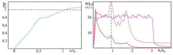
Figure 5a: Parabolic density profile with a MHD-like perturbation and extensive density fluctuations with an amplitude of 1 %
