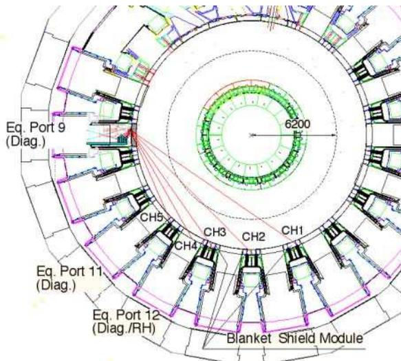
Fig. 3. Schematic plan view of lines of sight of the Interferometer/Polarimeter system on an equatorial port.
