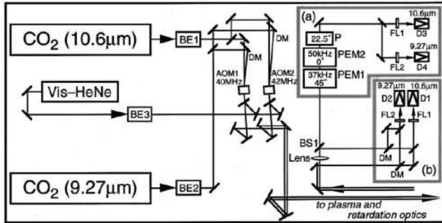
Fig. 1. Arrangement of the dual CO<sub>2</sub> laser interferometer / polarimeter on the optical bench of JT-60U.
