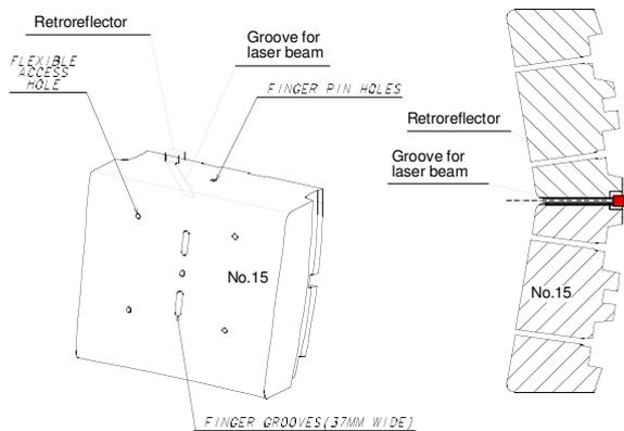
Fig. 5. Retroreflector placed behind the Blanket shield module.
