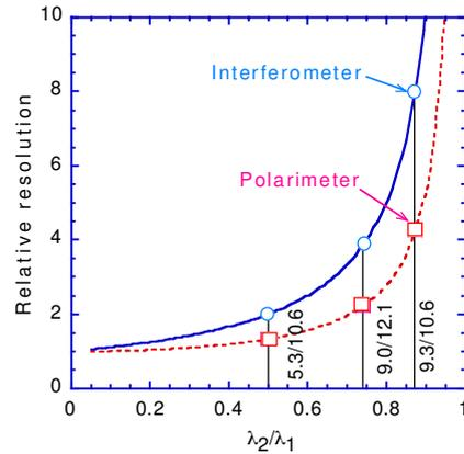
Fig. 2. Relative resolution for interferometry and polarimetry.
