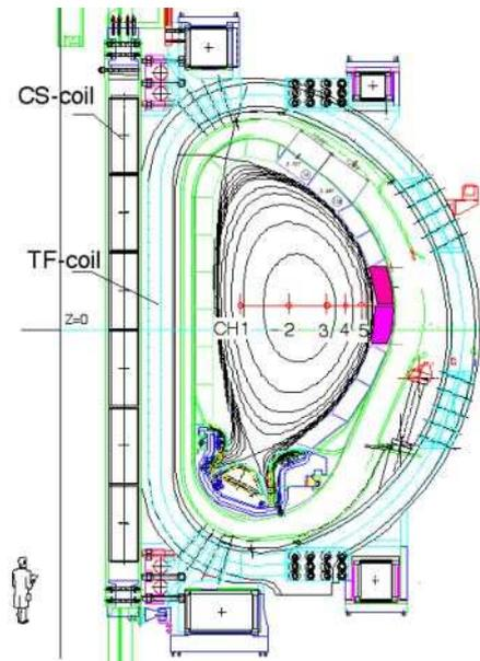
Fig. 4. Schematic sectional view of lines of sight.
