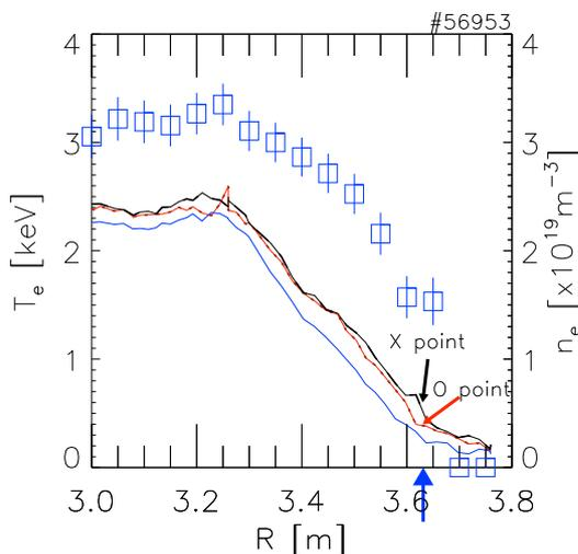
Figure 2:  $T_e$  ECE profiles (lines) and  $n_e$  LIDAR profile (squares). Profiles in blue were measured at 50.6276 s. In red and black at 50.6074 s and 50.6085 s, respectively (see black arrows in Fig. 1(a)). The red and black  $T_e$  profiles are shown to indicate the radius of the  $m/n = 2/1$  island. Just like in Fig. 1(a) the blue arrow indicates the position of the 76 GHz cut-off layer.
