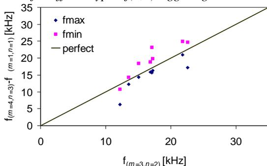
Figure 4: The difference between the frequency of the (4,3) mode and the minimum (pink) and maximum (blue) frequencies of the fishbone instabilities versus the frequency of the (3,2) NTM
