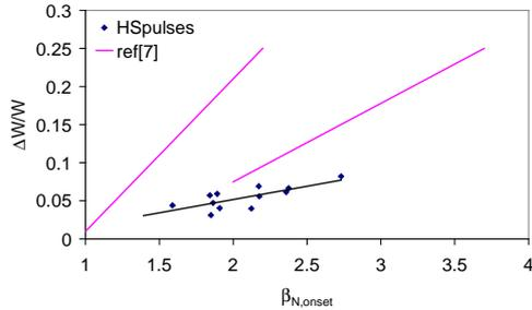
Figure 5: Relative confinement reduction (difference in plasma energy content at mode onset and after its saturation, normalised to the energy at NTM onset) due to (3,2) NTMs versus  $\beta_N$  at NTM onset for jet. The trend line in pink is for  $\beta_N > 0$  pulses from ref. [7].
