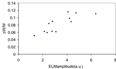
Figure 6: Relative confinement reduction (difference in plasma energy before and after the ELM, normalised to the energy before the ELM) due to single ELM
