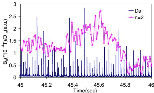
Figure 7: Radial perturbation of the magnetic field ( $W \propto \tilde{B}_r^2$ ) for (3,2) NTM and the  $D_\alpha$  signal for the pulse no: 60926
