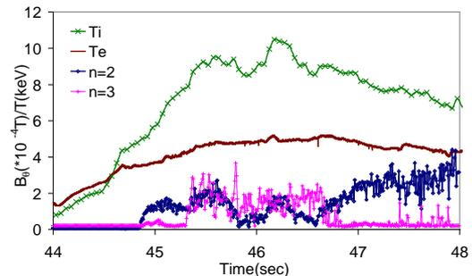
Figure 8: Mode amplitude for the (3,2) NTM (blue), 5\* the amplitude of the (4,3) NTM for comparison (pink); electron temperature at  $R = 3.2$  (brown); ion temperature at  $R = 3.14$  (green) for the pulse no: 60926
