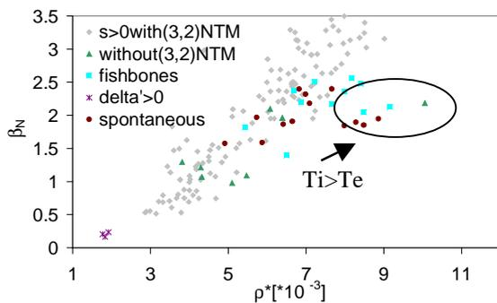
Figure 2:  $\beta_N$  versus  $\rho^*$  at the (3,2) NTM onset for HS pulses data base and without at the maximum value of  $\beta_N$  and pulses with (3,2) NTM for  $s > 0$
