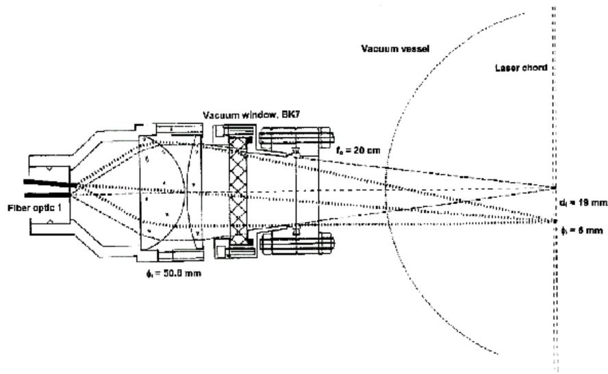
Fig. 2: Collection optics made of plan convex and an aspherical lens and two optical fibre with 1,5 mm diameter.
