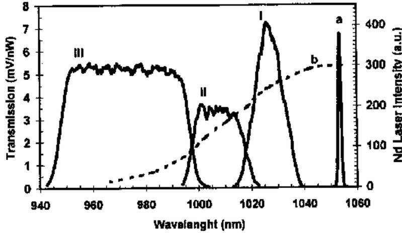
Fig. 3: Spectrometer Calibration. Curves I, II and III are the calibration curves of each interference filter. Curve (a) its the natural broadening of the Nd-Glass laser line. Curve (b) its the Doppler broadening laser line in a plasma with  $T_e = 250$  eV and  $n_e = 1 \times 10^{18} \text{ m}^{-3}$ .
