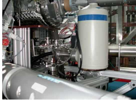
Figure 7.1 – View of the horizontal PHA diagnostic on TCV
