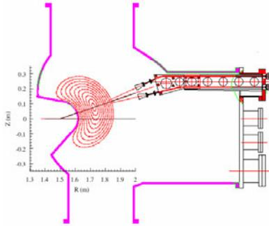
Figure 5.2 - Arrangement of the antennas and waveguides inside the vacuum vessel and magnetic surfaces of the standard magnetic configuration.
