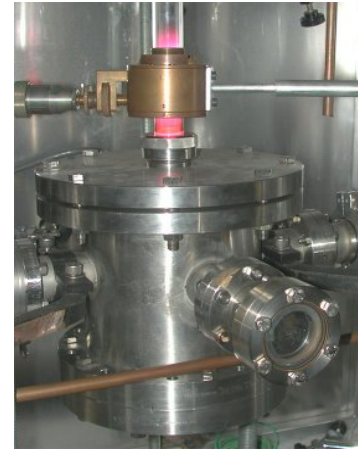
Figure 13.20 – Microwave reactor (cylindrical configuration), (ICMS, Sevilla, Spain).
