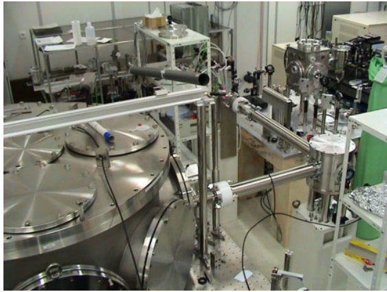
Figure 11.3 – View of new in-vacuum beam delivery system
