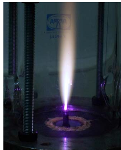
Figure 1.5 - Plasma torch, developed at the University of Cordoba (Spain), and modeled at CFP.
