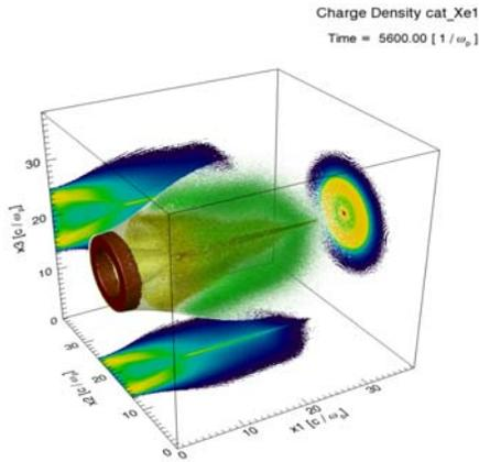
Figure 13.12 - Xe+ ions originating from the thruster. The thruster plume pinches after a stage of free expansion leading to higher flow velocity. Densities [ $e \omega_{03c3}$ ]: red 1, yellow 0.3 and green 0.1.
