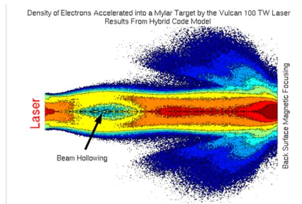
Figure 13.1 - Results from hybrid code modelling of experiments on the Vulcan 100 TW laser with solid, plastic targets (Mylar) that reproduces the electron beam hollowing.
