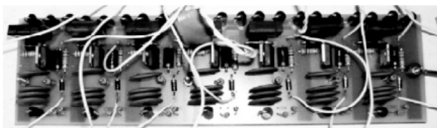
Figure 14.12 - MOSFET switch module, showing 7 MOSFET units. The main MOSFET is seen on top, and part of the protection and driving circuitry is directly below
