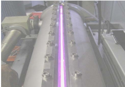
Figure 18.4 - Coaxial microwave plasma reactor with the LPGP (Orsay, France).
