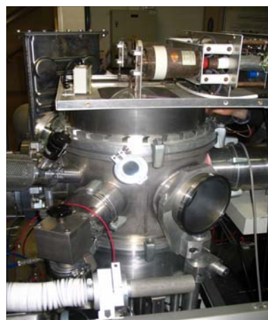
Figure 18.1 - ICP reactor with the LPCM (Nantes, France)
