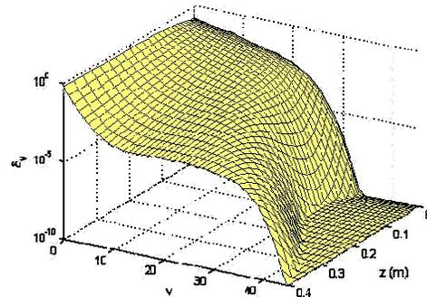
Figure 16.1 - Axial variation of the vibrational distribution function (80%N<sub>2</sub> – 20% Ar, *p* = 0.9 mbar, *r* = cm, φ = 162).
