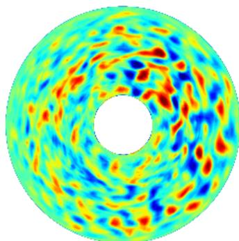
Turbulent  $\delta n$  on poloidal cross section.
