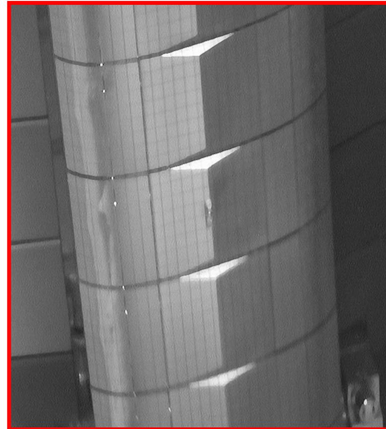
A slide-away event caused the first melt damage, within 100 plasma pulses from first plasma.
