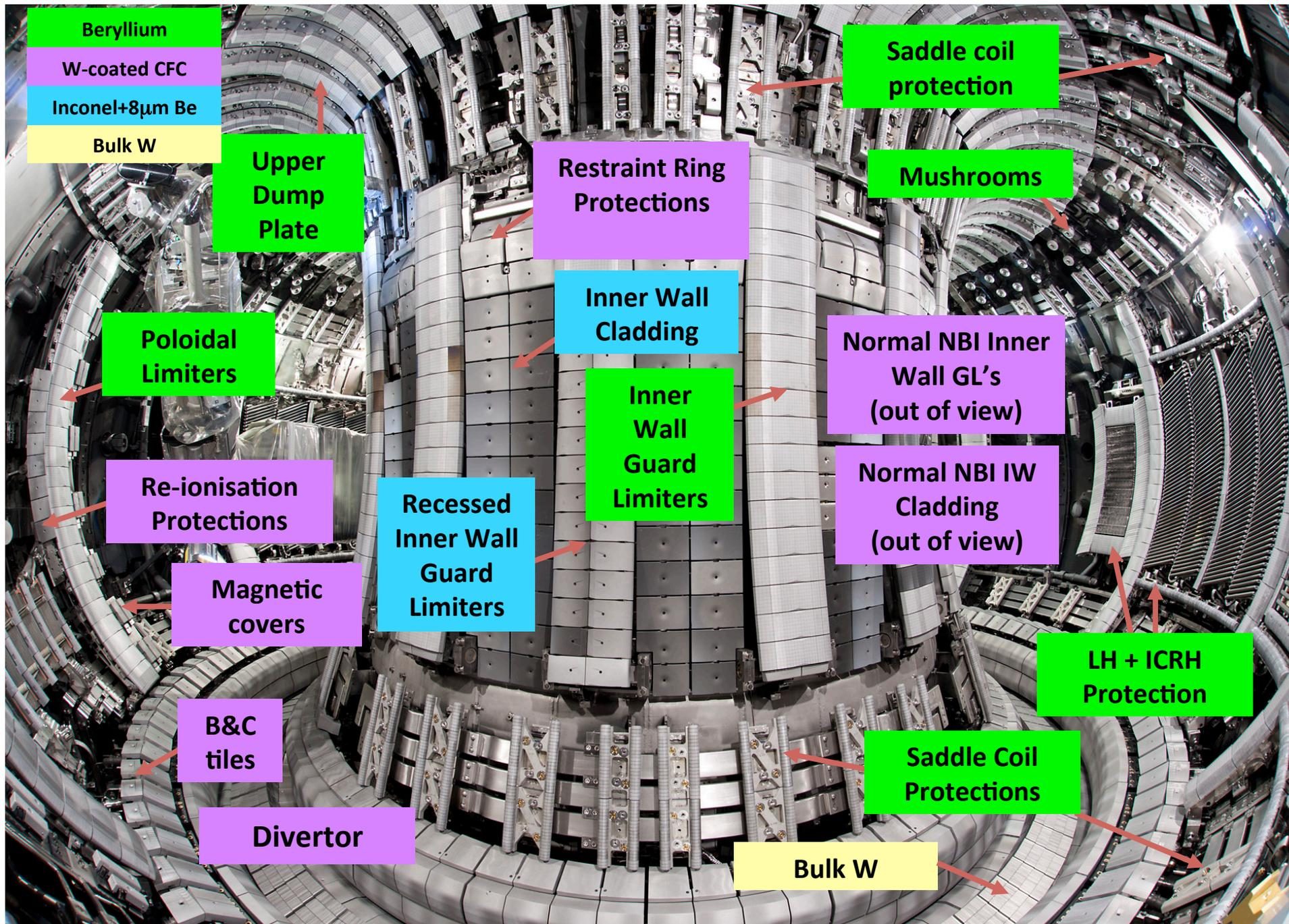
**ILW = 2880 installable items, 15828 tiles (~2 tonnes Be, ~2 tonnes W)**
