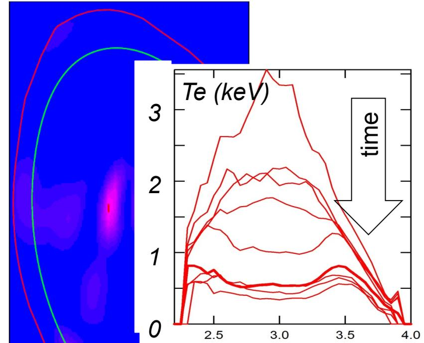
*Progressive increase of radiation on central chords from ~49s → core temperature collapse ~51s, and build up of radiation*
