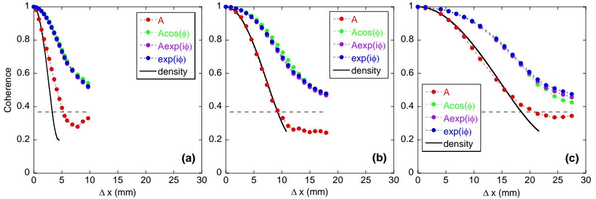
Figure 1. Coherence of different reflectometry signals in linear regime: amplitude (red), homodyne (green), complex amplitude (purple) and complex phase (blue) as a function of layer separation. The results are shown for radial correlation lengths (a)  $l_{cx} / \lambda_0 \approx 0.4$  ( $\gamma = 0.07$ ), (b)  $l_{cx} / \lambda_0 \approx 1.2$  ( $\gamma = 0.13$ ) and (c)  $l_{cx} / \lambda_0 \approx 2.5$  ( $\gamma = 0.18$ ). The solid line represents the coherence of density fluctuations.
