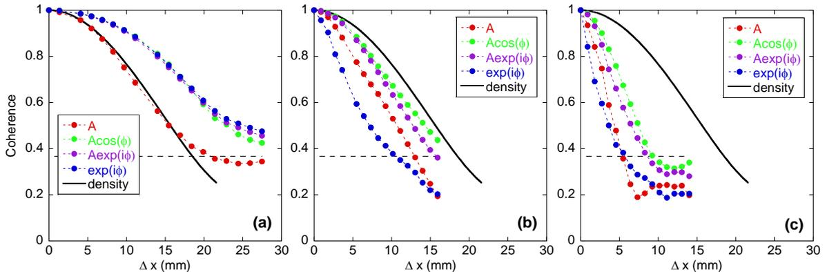
Figure 2. Coherence of amplitude, homodyne, complex amplitude, and complex phase signals as a function of layer separation. The results are shown for three turbulence level (a)  $\delta n_{rms}/n = 1\%$  ( $\gamma = 0.18$ ), (b)  $\delta n_{rms}/n = 5\%$  ( $\gamma = 4.62$ ), and (c)  $\delta n_{rms}/n = 10\%$  ( $\gamma = 18.49$ ). The solid line represents the coherence of density fluctuations.
