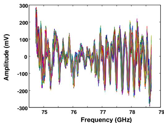
*Figure 3 : Test for stability of the reflectometers by a superposition of 1000 signals reflected on mirror (beginning of the V-band reflectometer). The burst mode conditions are : sweep time  $4 \mu s$  dead time =  $1 \mu s$ .*
