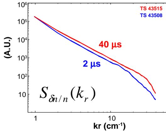
**Figure 5 : Experimental wavenumber density fluctuation spectrum record on similar ohmic plasma discharges**
