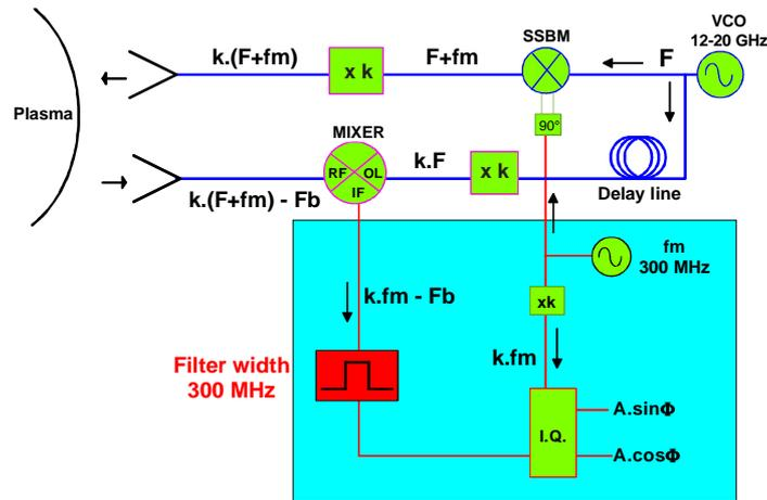
*Figure 2 : Schematic of the reflectometers (with  $k = 4$  and  $6$  respectively for the V and W bands). The blue area is related to the IF part which has been mostly renewed to account for the beat frequency ( $F_b$ ) range increase.*
