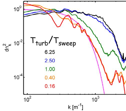
**Figure 4 : Numerical simulation of the wave number fluctuation spectrum modification with respect to the sweep time with the input spectrum (magneta).**
