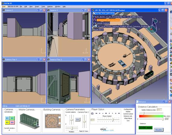
Fig. 10. Virtual Reality system developed by ASTRIUM ST for operation supervision of remote handling operations of transportation under the grant F4E-2008-GRT-016 leaded by IST.
