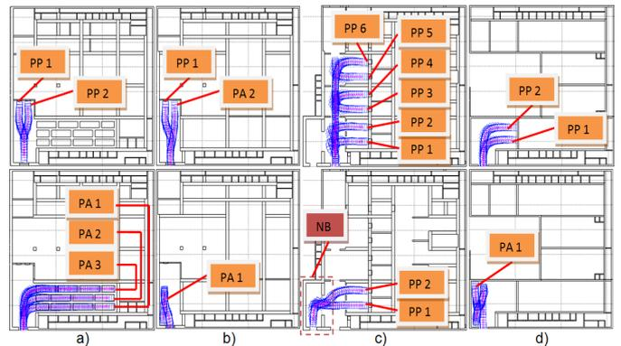
Fig. 7. Set of all trajectories in HCB. In a): level B2; b): level B1; c): level L1; d): level L3. Top: docking locations; Bottom: parking locations (same path for both wheels).
