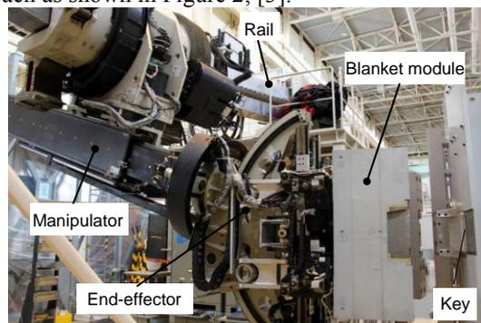
Fig.2. Installation of a blanket module.
