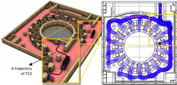
Fig.6. Trajectories of the TCS in the divertor level of TB.
