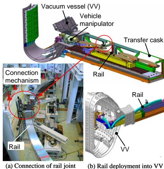
Fig.1. Demonstration of the rail joint connection.
