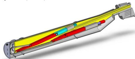
Fig.8. Schematic view of the IVVS-GDC plug (IVVS grey-blue probe in upper position, VV entrance on the right).
