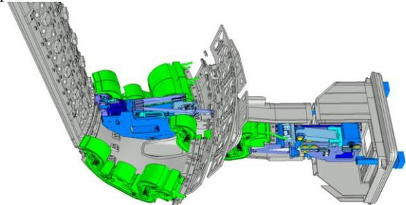
Fig.3. Sketch of the Divertor RH System in operation.
