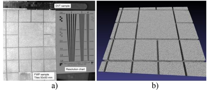
Fig.10. a) Viewing image taken by the IVVS; b) 3D image, in STL format, produced by the IVVS.
