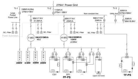
Figure 1: The proposed AC power supply system in JT-60SA (Initial experimental phase)
