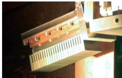
Prototype stack of solid tungsten lamellae in the MARION facility before exposure (stack length: 165 mm)
