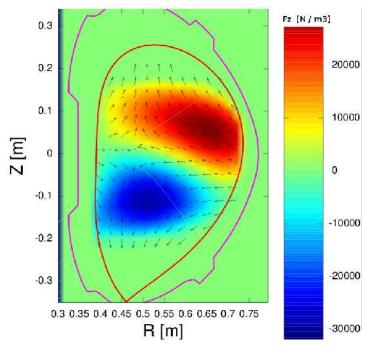
Poloidal cross-section of plasma in the COMPASS tokamak shows how the volumetric magnetic force (red upwards, blue downwards) stretches the plasma vertically, as desired, but also yielding vertical instability. For typical conditions, the force is a product of toroidal plasma current density and poloidal magnetic field.
