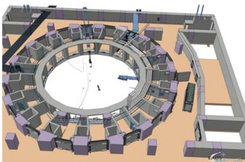
Figure 1: 3D VM of the Tokamak building divertor (level B1) with the CPRHS during a nominal operation
