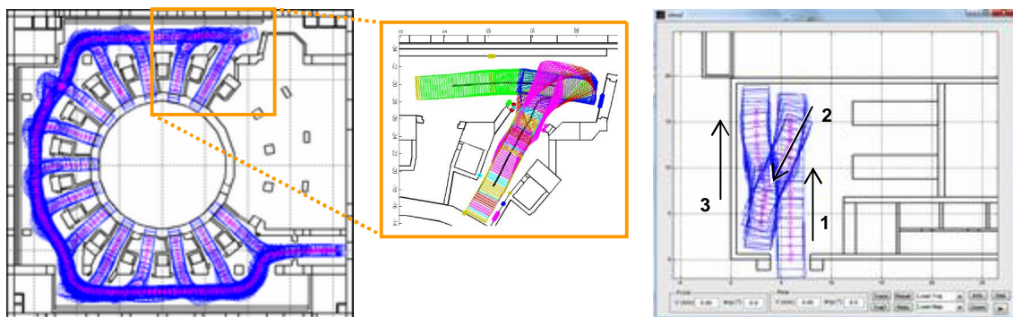
Figure 1 – (left) the 14 optimized trajectories in level L1 of TB; (center) maneuver in the entrance of Vacuum Vessel port cell number 8; (right) parking maneuver in level L3 of HCB.
