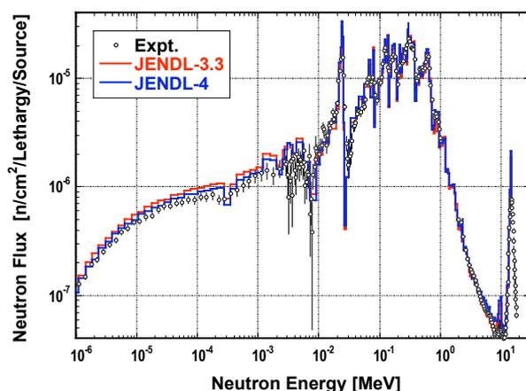
Figure 1: Neutron spectra at 41 cm inside iron assembly
